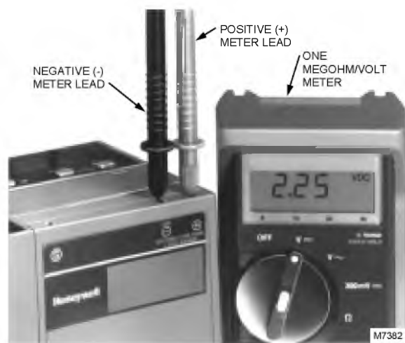
Fig. 13—Measuring 7800 SERIES controls flame signal voltage.
