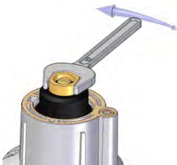
Figure 24: Adjusting flow rate.
