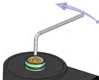
Figure 22: Adjusting flow rate.
